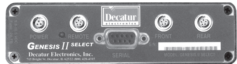
Figure 4b The Genesis II Select rear interface
