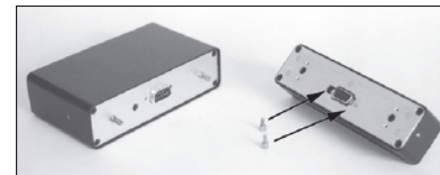
Figure 2.1b To connect the separated unit, first insert the standoffs to secure the cable connectors.
