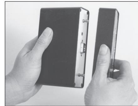
Figure 2.1a Separating the computer/display unit.
